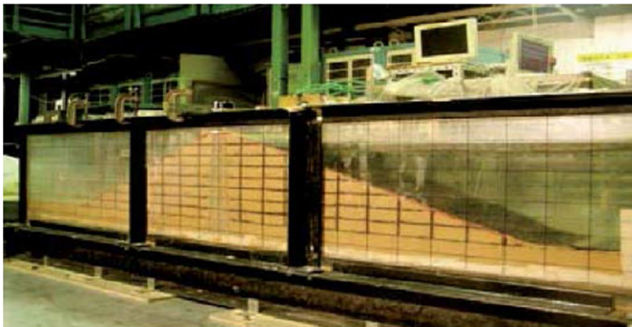
Fig. 45 An embankment with the reservoir on a shaking table test (Torisu et al. 2010)
