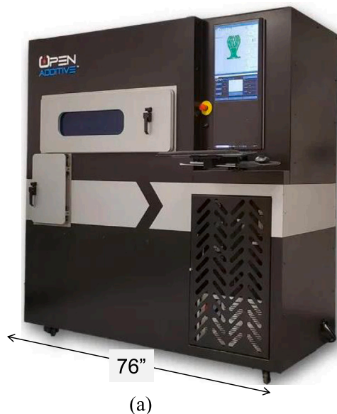
Fig. 12. (a) PANDA 11 open architecture LPBF machine; and (b) fixture used for positioning plates during scanning experiments. The plates sat on the four insulating washers within the 6.2\text{ cm} \times 6.2\text{ cm} opening of the frame.
